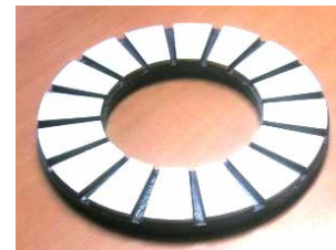
Fig 7. Design of stator and rotor of axial flux permanent magnet motor
