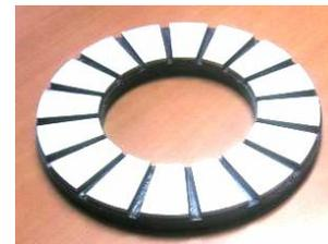
Fig 8. Assembly of permanent magnet and Rotor Back Iron of Axial Flux Permanent Magnet Motor
